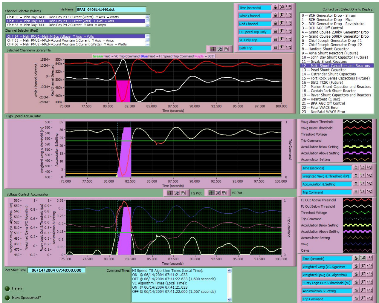
Figure 9: WACS development PC computer plots for capacitor/reactor bank switching using June 14, 2004 archived data. The top plot shows selected representative input signals. The white channel is John Day PH Line 1 reactive power; negative is into the John Day switchyard. The red channel is Malin voltage. On the upper right, the selection of contact 12 for Malin shunt capacitors and reactors means that the middle and lower plots are for capacitor/reactor bank switching. The middle plot is for the voltage magnitude based algorithm. The white/red signal is the weighted average voltage (turns red when below threshold for volt-second accumulation). The green line is the threshold (525 kV). The yellow and purple signals are the accumulated volt-seconds, and the orange line is the accumulator setpoint; the small yellow area is the volt-second area to initiate control action (dashed blue line). The lower plot is for the voltage magnitude, generator reactive power fuzzy logic algorithm. The blue and orange signals are the weighted average voltage and weighted average reactive power inputs to fuzzy logic. The white/red signal is the fuzzy logic per unit crisp output (turns red when above threshold for per unit-second accumulation), and the green line is the accumulator setpoint (0.5 per unit). The yellow and purple signals are the accumulated per unit-seconds, and the orange line is the accumulator setpoint; the small yellow area is the per unit-second area to initiate control action (dashed blue line). The lower blue box gives WACS operation times.
