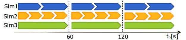
Fig. 1. An example of a co-simulation involving three simulators: *Sim1*, *Sim2*, and *Sim3*, with a step size of 30, 15, 60 seconds, respectively.
